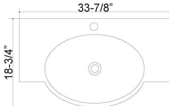
Dimensions of fixture are nominal and may vary within the range of tolerances established by ASME Standard A112.19.2.2013. Dimensions and specifications subject to change without notice.
