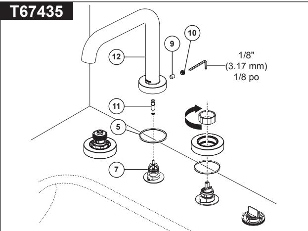
**NOTE:** The deck and valve rough-in (R62707 for T67335 and R64707 for T67435) must be finished before installing the trim kit.
