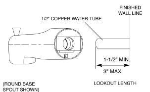
Lookout must be free from deep scratches, dents, kinks or bends. The cut-off end must be free from burrs inside and out. The edge must not be rolled inward from a dull tubing cutter.
