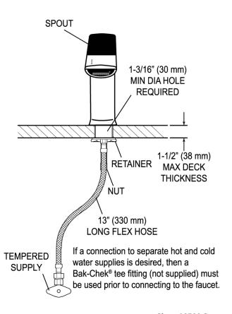
Solenoid valve housed in removable carrier that closes water supply upon removal eliminating, need to access control stops. Solenoid carrier includes strainer for easy above deck service. Thermostatic mixer ordered separately to comply with ASSE 1070 requirements. The product shall be tested and certified to industry standards: ASME A112.18.1M, CSA B125.1, California Health and Safety Code 116875
