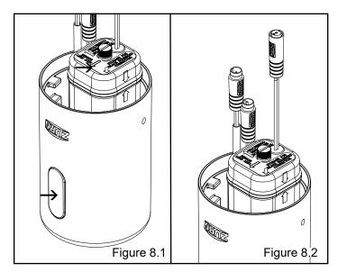
STEP 5A.3 Reattach the sensor cap and tighten cap screws.
