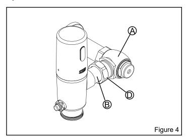
⚠ **DO NOT** use pipe sealant or plumbing grease on any valve component or coupling with the exception of the Control Stop Inlet! Ensure Vacuum Breaker does not twist or warp when tightening Vacuum Breaker Tube Nut.
