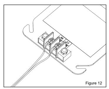
Optional Junction Box (recommended when three or more ZTR flush valves utilize one HW6)
